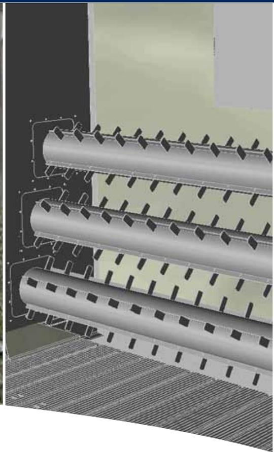
De-compacting/cutting unit for silage
