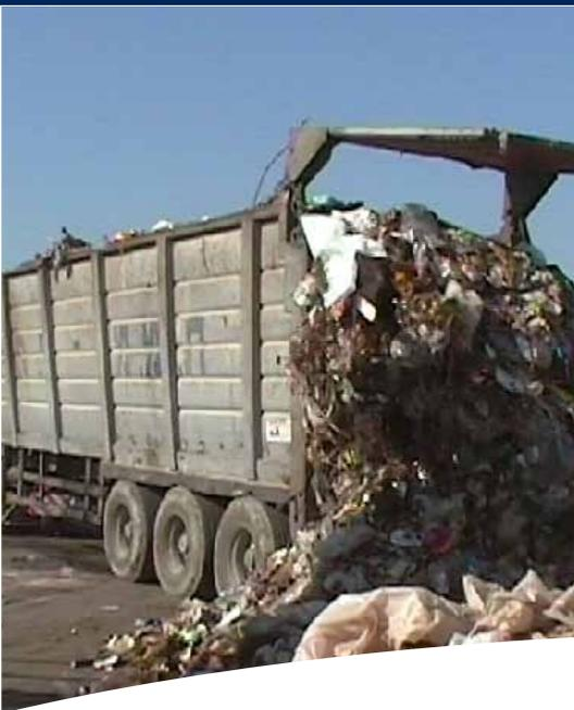
*Heavy impact floor to transport and offload
