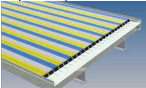
*Aluminium floor profiles are driven in three groups to achieve an endless movement cycle*
