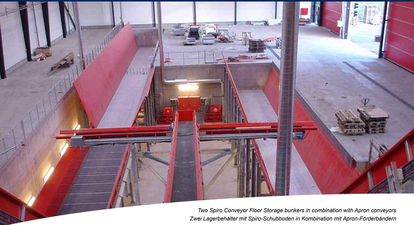
*Two Spiro Conveyor Floor Storage bunkers in combination with Apron conveyors
